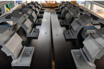
Boyce has been experiencing the benefits of 3D printing in reducing costs and bringing products to market faster. Parts can be made to exacting specifications without outsourcing the work, reducing costs and time to have parts in hand. Furthermore, unlike injection molding, costly tooling is not required when creating end-use parts, so there's no hold-up when a design is ready for production.
