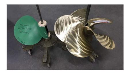
A typical pattern print for a 750mm long design takes just 40 hours to print. Total production time is just 48 hours when including post-processing work. That two days means a 33% faster pattern production time, cut down from three days. A 90% reduction in pattern maker costs further highlights the benefits of bringing large-format 3D printing in-house.
