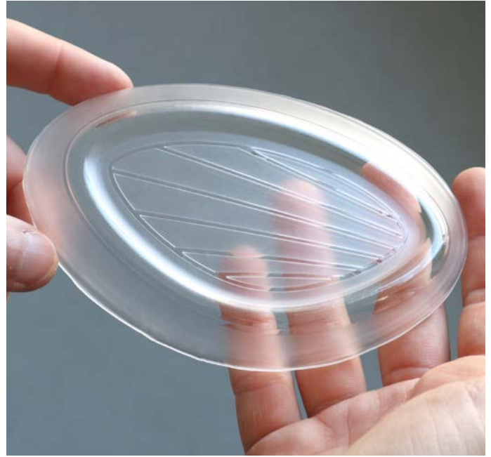
Car light lens made on the Mayku Multiplier.
